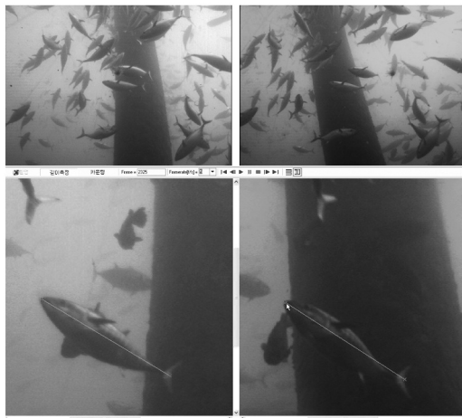
Fig. 9. Captured pictures (upper) and fish size measured pictures (down) of stereo camera system.
