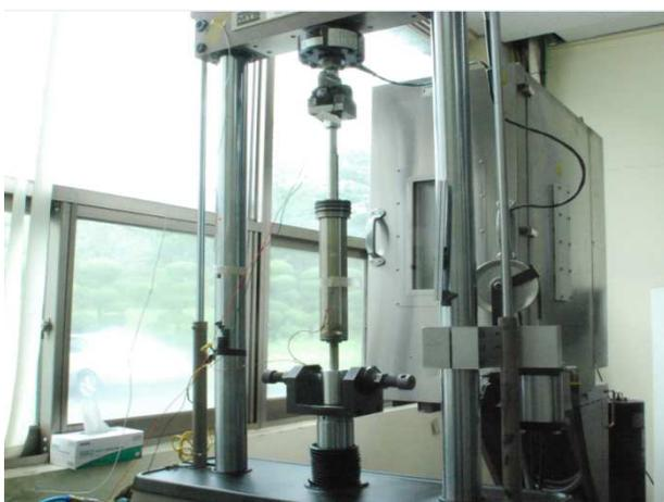
**Fig. 1** Characteristics test of MR damper
