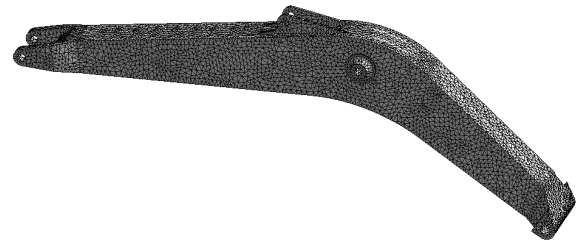
Fig. 2 Finite element model of boom structure
