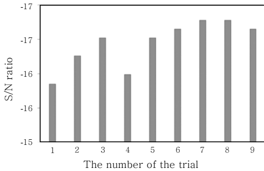
Fig. 10 S/N ratio of the bead width
