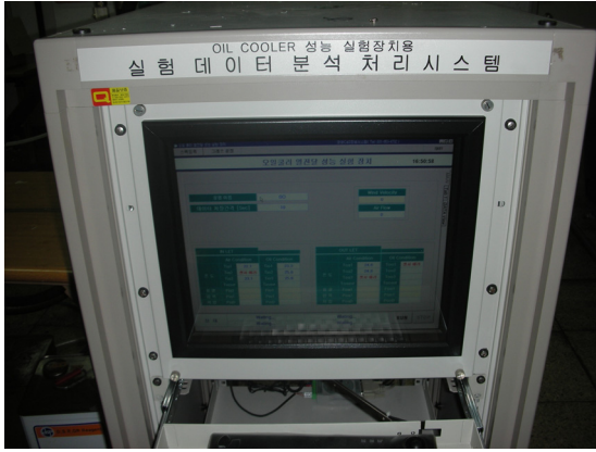
Fig. 4 Data acquisition system
