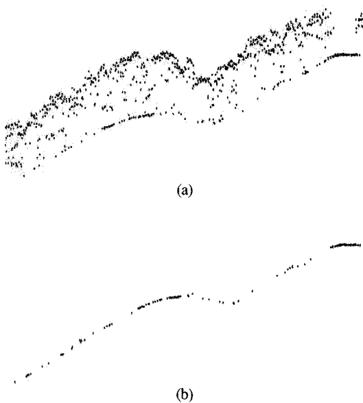
Fig. 3. (a) LiDAR data in forest areas. (b) Ground points classified after filtering.
