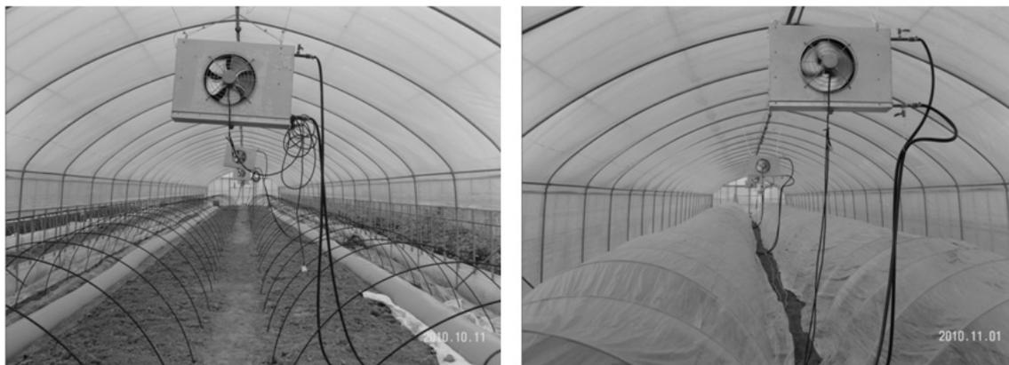
Fig. 2 Experimental greenhouse with FCU.
