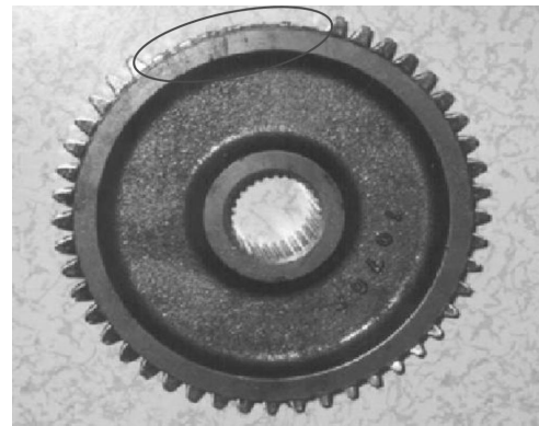
Fig. 5 Photo of the broken PTO driving gear by the fatigue life test.
