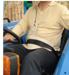
Figure 4. Measuring the body pressure while wearing manual seatbelt
