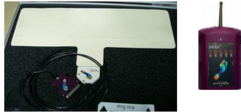
Figure 1. Measurement instrument of body pressure distribution
