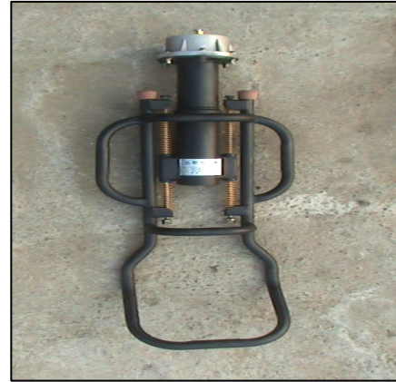
Figure 2. Example of Pile Driver
