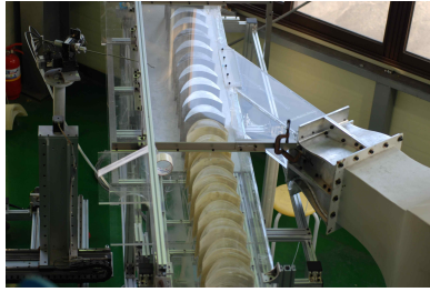
Fig. 2. Picture of the linear cascade apparatus
