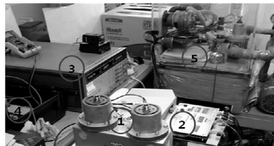
Fig. 2. Capacitance measuring devices: ①-Filter-sensor, ②-Sensor controller & monitoring system, ③-Impedance analyzer, ④-Data logger, and ⑤-Engine lubrication system rig tester.
