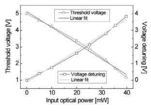
Fig. 6. Tuning linearity of the threshold voltage and voltage detuning of the  $VO_2$  device.
