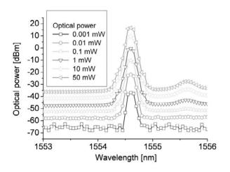
Fig. 4. Measured optical power spectra of EDFA output.
