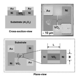
Fig. 1. Cross-section and plane-views of the fabricated VO<sub>2</sub> device and its plane-view optical microscope image(upper right corner).
