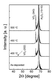
Fig. 2. XRD patterns of VO<sub>2</sub> films grown on Al<sub>2</sub>O<sub>3</sub>(10-10) substrates. The films were annealed at various temperatures in an oxygen atmosphere of 32 mTorr.
