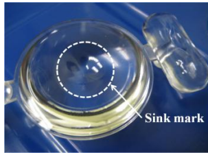
Fig. 6 A sink mark phenomenon shown on the upper surface of injection molded lens
