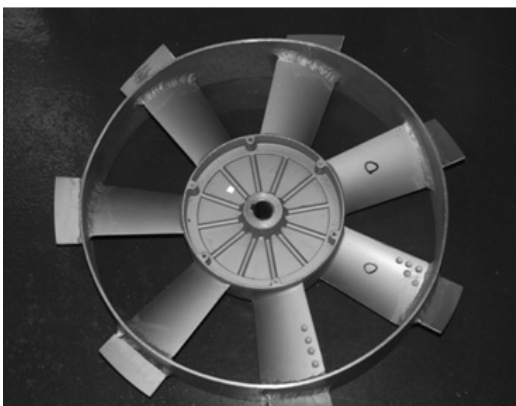
Fig. 3 Picture of a suction-blowing fan rotor
