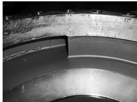
Fig. 11 Crack at the fuel pump volute
