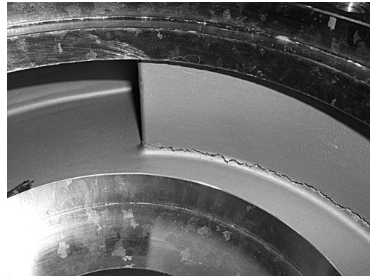
Fig. 10 Crack at the oxidizer pump volute
