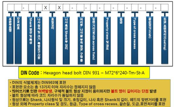
Fig. 8. Analysis of DIN962
