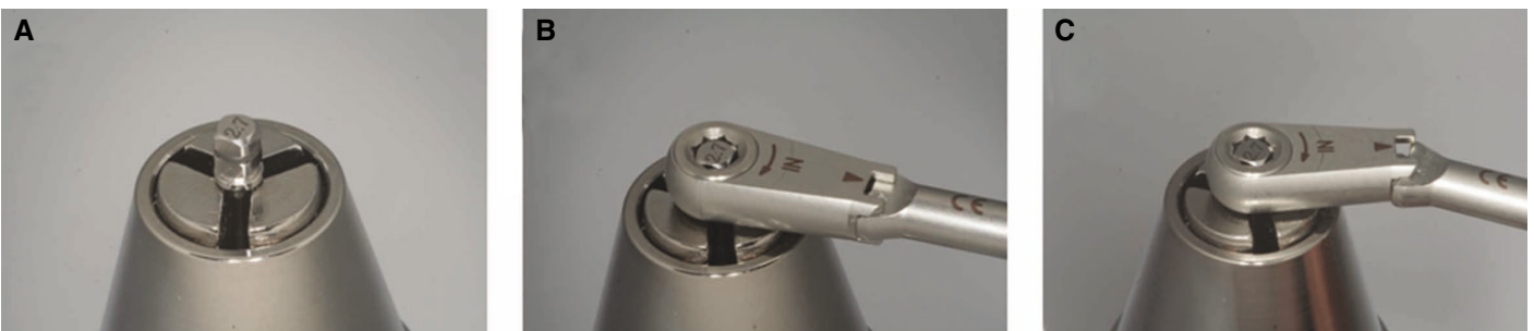
Fig. 3. Torque controller accuracy test (A: square insert in the jaws of the Tonichi Torque Gauge, B: torque controller under test condition, C: torque controller is rotated until the detent releases).
