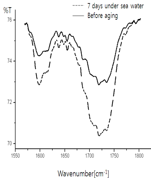
Figure 7. IR spectra of PUF from aliphatic polyether polyol under sea water.
