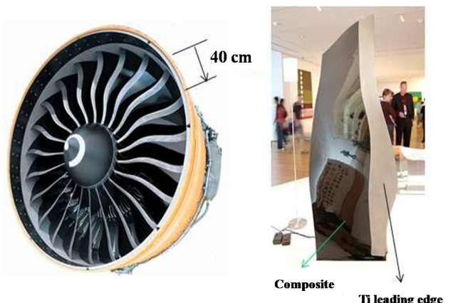
Figure 3. Composite fan blade for B787 engine(GE90).
