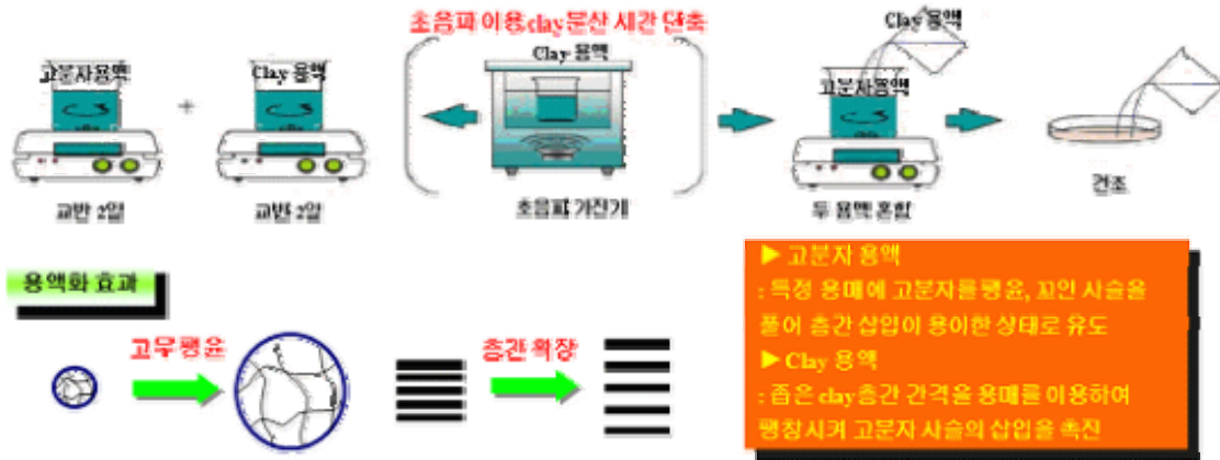
Figure 13. Schematic of nanocomposite preparation by solution method.
