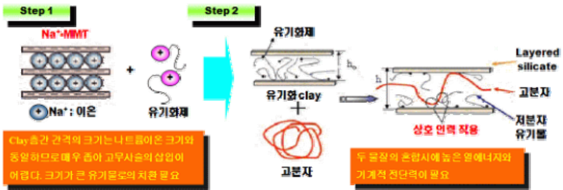
Figure 14. Schematic of nanocomposite preparation by the compounding method.
