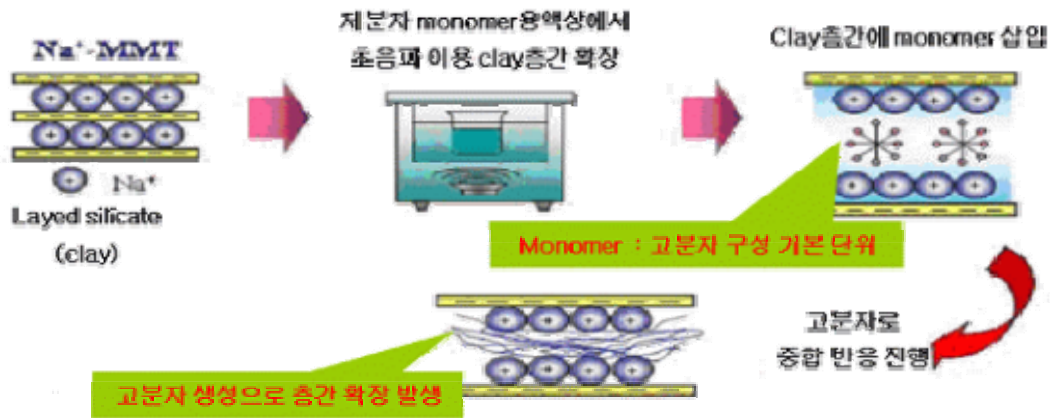
Figure 12. Schematic of nanocomposite by the polymerization preparation method.
