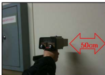
Fig. 3. Measurement of leakage dose in the wall
