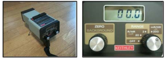
Fig. 1. Keithley integrating radiation survey meter (model 36150). This survey meter used in various applications of radiation surveys were placed at the same distance from the center of the scattering material.
