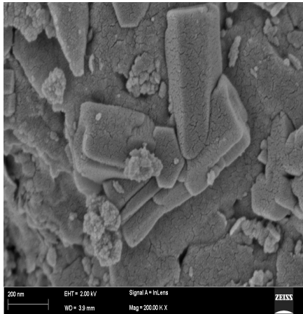
(b) Coal mine drainage sludge+cement+bentonite(x 200,000)
