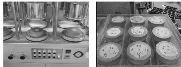
a) water permeability test b) Water absorption coefficient
