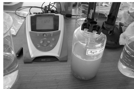
Fig. 5 pH test of recycled aggregate by pH meter
