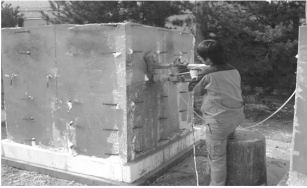
Fig. 2 Coring scene of mock-up specimen
