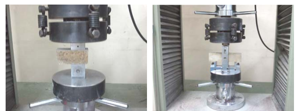
Fig. 4 Compressive and bending strength test
