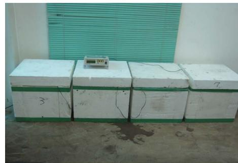
Fig. 4 Hydration heat measurement
