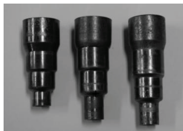
Fig.11 Products of forging at each stage
