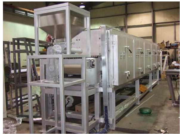
Fig. 2 Industrial dryer with catalytic burners; (a) schematic diagram; (b) photograph
