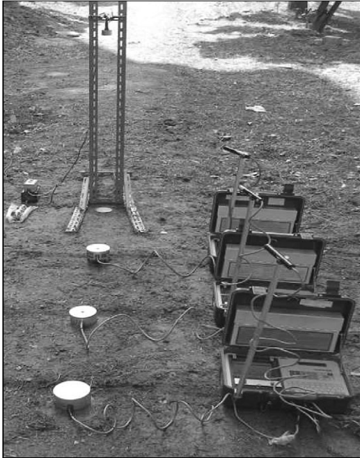
Figure 1. Image of Shock Vibration Test Device
