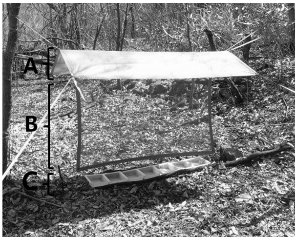
Fig. 2. Flight Interception Trap (FIT) in Beopjusa. A: roof; B: vertical screen; C: collecting container.
