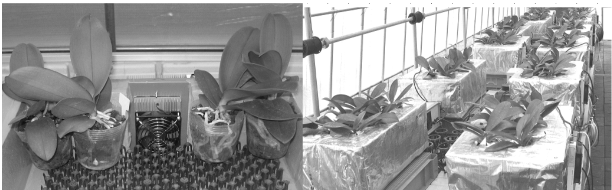
Fig. 1. Root zone temperature control system of Peltier device used in this experiment.
