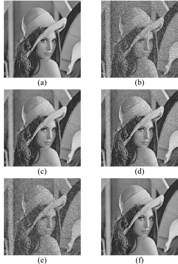
Fig. 2. Simulation results. (a) Test image (b) Noisy image (c) SM ( 3 \times 3 ) (d) CWM ( 3 \times 3, C=3 ) (e) MF ( 3 \times 3 ) (f) Proposed filter
