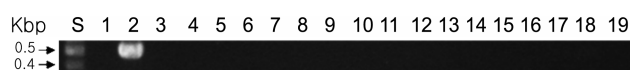
Fig. 2. Specificity test of the Pig28-F1/Pig28-R1 primers using 2 ng of each bacterial of the clinical isolates of P. intermedia and P. nigrescens . The PCR reaction products were electrophoresed on 1.5% agarose gel. Lanes: S, size marker (100 bp ladder); 1, (-) negative control; 2, P. intermedia ATCC 49046; 3, P. intermedia KCOM 1101; 4, P. intermedia KCOM 2671; 5, P. intermedia KCOM 1104; 6, P. intermedia KCOM 1106; 7, P. intermedia KCOM 1107; 8, P. intermedia KCOM 1109; 9, P. nigrescens KCOM 1032; 10, P. nigrescens KCOM 1034; 11, P. nigrescens KCOM 1036; 12, P. nigrescens KCOM 1040; 13, P. nigrescens KCOM 1041; 14, P. nigrescens KCOM 1042; 15, P. nigrescens KCOM 1044; 16, P. nigrescens KCOM 1102; 17, P. nigrescens KCOM 1103; 18, P. nigrescens KCOM 1108.
