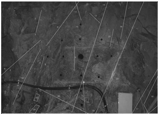
Fig. 2. Boreholes for in situ heater test and joints around the test area
