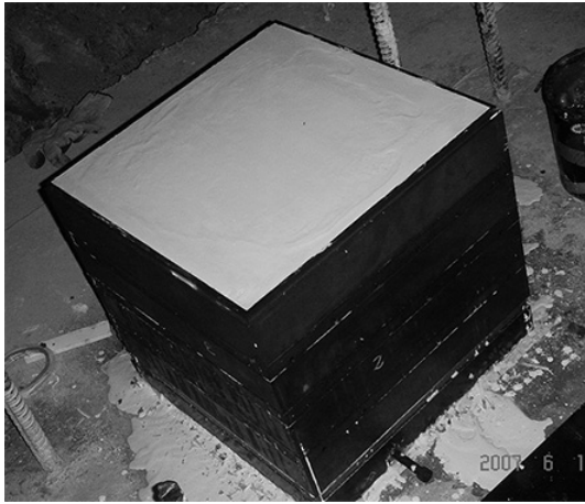
Fig. 7. Molding shear box on the test block
