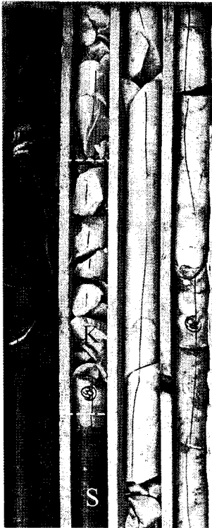
Fig. 5. The Geumseong magnesian skarn(S)-cupola(C) contact aureole showing sampling site in K-feldspar zone (K) (drill hole GSM2006-3; ca. 260m). K-feldspar caps developed as a result of fractionation at the upper portions of a Mo-bearing cupola.
