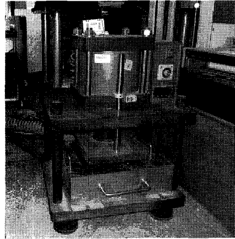
Figure 1. Laboratory installation damage test equipment.
