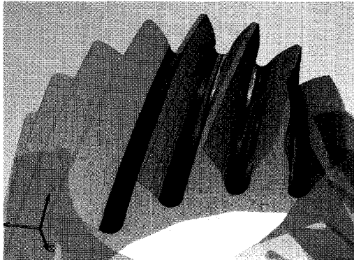
Fig. 3 Bending stress distribution at tooth roots of the sun gear
