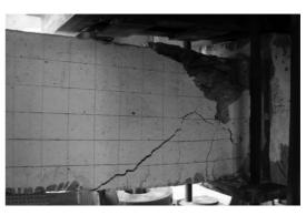
Fig. 7 Damage pattern of Specimen D4 at center column (*P* = 53.5 kN).
