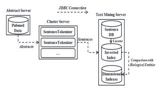
Figure 6. Data processing procedure for sentence tokenizing and dimensional indexing. The procedure consists of three steps: the first step is to get abstracts from the local PubMed database; the second step is to tokenize and deliver the sentences to the text mining server; the third step is to make dimensional indexes for biological entities. As the data delivery is performed only on network, additional works in each node of the cluster system are unnecessary.
