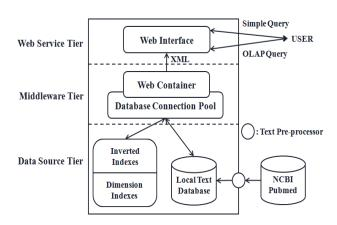
Figure 5. PubMine architecture. PubMine consists of three tiers: a data source tier, a middleware tier and a web service tier. The data source tier manages original text data and related indexes (dimension indexes and inverted index). The middleware tier provides an application server for java servlets and database pooling. Finally, the web service tier provides a user-friendly web interface including an easy query window for simple and OLAP searches.
