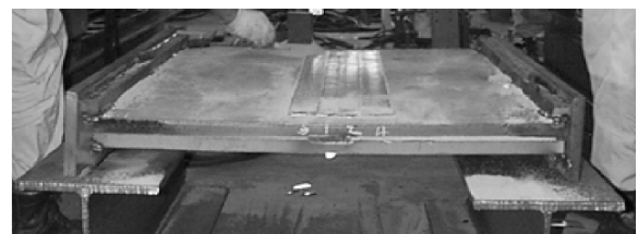
(a) front side 1 layer welding
