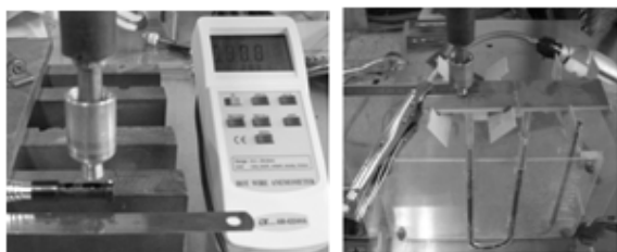
a) Gas velocity test b) Gas pressure test
