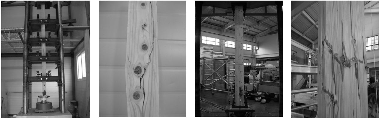
Fig. 3. Compressive strength test of specimens.
