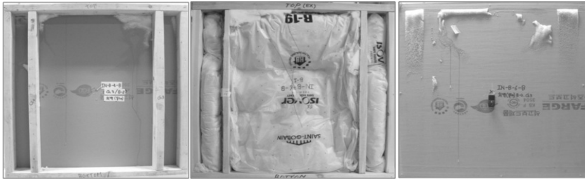
Fig. 6. Failure mode of B-B wall systems.
