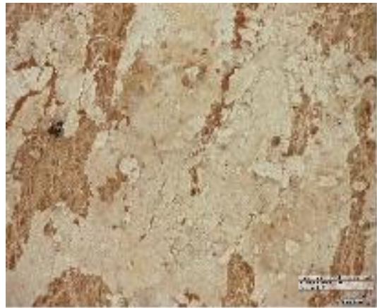
Figure 4. Results of video microscope for layers of white pigment.
