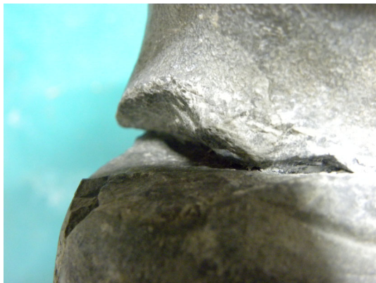
Figure 13. Filling material state of the shoulder part in xylene after 2 hours.
