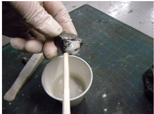
Figure 4. Apply the urethane to adhesion part.
