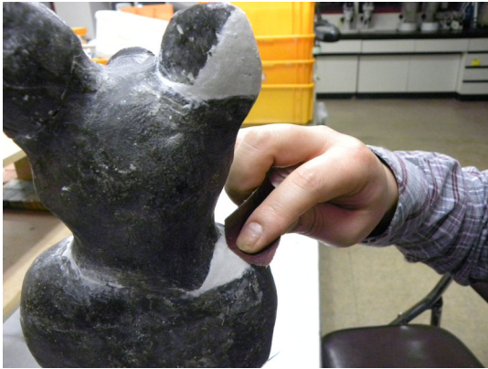
Figure 9. Surface arrangement with sand paper.
