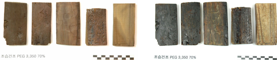
Figure 12. Humidity-controlled dried samples(pretreatment: PEG 70%; HCD70; left-before drying, right-after drying).
