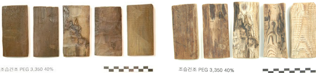
Figure 9. Humidity-controlled dried samples(pretreatment: PEG 40%; HCD40; left-before drying, right-after drying).
