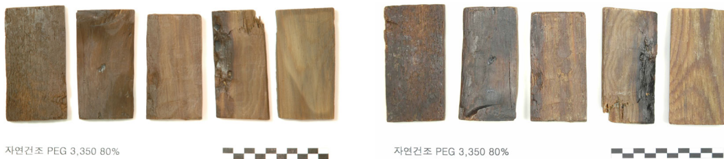
Figure 13. Natural dried samples(pretreatment: PEG 80%; HCD80; left-before drying, right-after drying).
