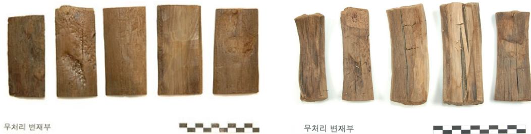
Figure 7. Natural dried samples(untreatment: ND00; left-before drying, right-after drying).
