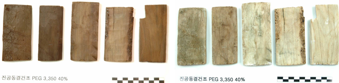
Figure 8. Vacuum freeze dried samples(pretreatment: PEG 40%; VFD40; left-before drying, right-after drying).
