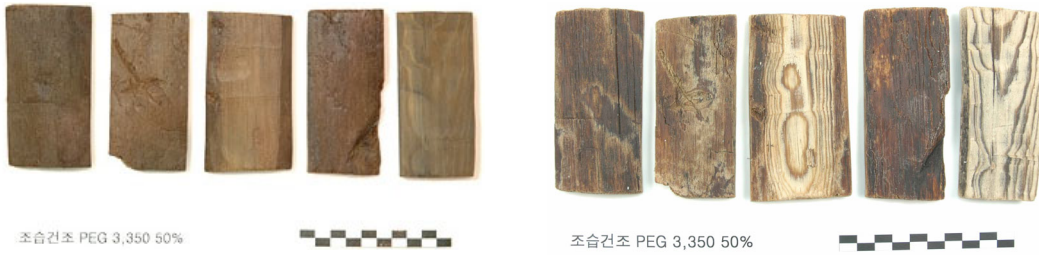
Figure 10. Humidity-controlled dried samples(pretreatment: PEG 50%; HCD50; left-before drying, right-after drying).
