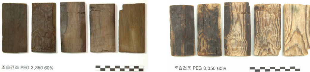
Figure 11. Humidity-controlled dried samples(pretreatment: PEG 60%; HCD60; left-before drying, right-after drying).
