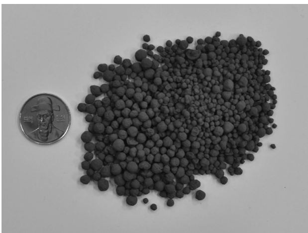
Fig. 2. Picture of the carbon based adsorption catalyst. The carbon content is 35%.
